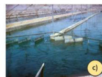
PBRs and raceways in operation in partners units: a) Tubular PBR in A4F microalgae production unit, Portugal; b) Green Wall Panels of F&M, Italy; c) and d) Raceways of 2000 m 2 , designed by BCU and in operation at Ein Yahav, Israel.
