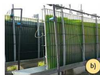
PBRs and raceways in operation in partners units: a) Tubular PBR in A4F microalgae production unit, Portugal; b) Green Wall Panels of F&M, Italy; c) and d) Raceways of 2000 m 2 , designed by BCU and in operation at Ein Yahav, Israel.
