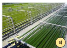
PBRs and raceways in operation in partners units: a) Tubular PBR in A4F microalgae production unit, Portugal; b) Green Wall Panels of F&M, Italy; c) and d) Raceways of 2000 m 2 , designed by BCU and in operation at Ein Yahav, Israel.
